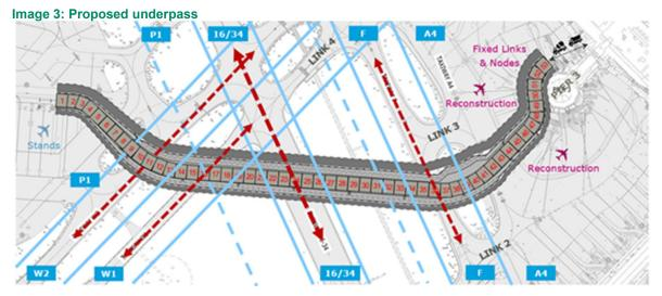
The proposed eastern portal is entered via a ramp which wraps around the north of Pier 3, before descending into the enclosed tunnel section.
